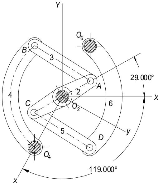
6. Determine the angular velocity of links 3 and 4 for the crossed circuit using equations 6.18.
