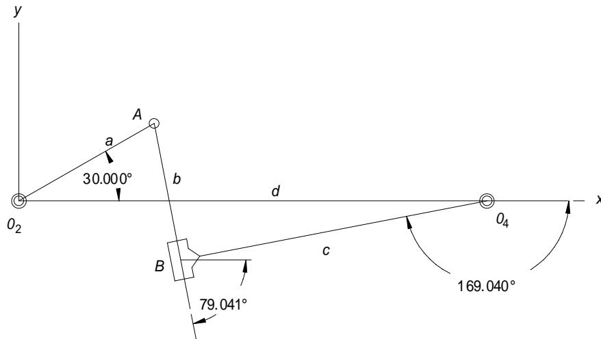
2. Use the equations in Section 4.7 to solve for the positions of links 3 and 4 and for the length *b*.
