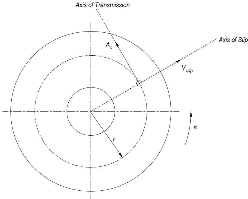
2. The direction of your path defines the axis of slip. The transmission axis is perpendicular to the axis of slip and positive in the direction of the tangential velocity of the carousel. Thus, the direction of the Coriolis acceleration vector is along the positive transmission axis.
