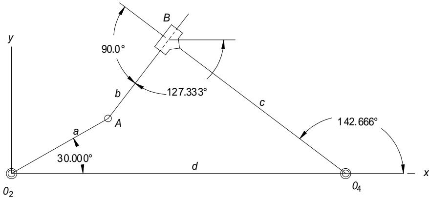
2. Use the equations in Section 4.7 to solve for the positions of links 3 and 4 and for the length *b*.
