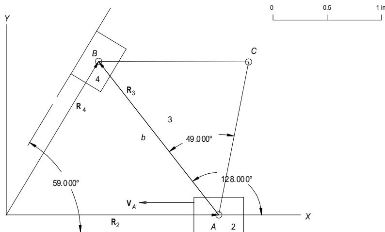
2. Write the vector loop equation, differentiate it, expand the result and separate into real and imaginary parts to solve for  $\omega_3$  and  $\mathbf{V}_B$ .
